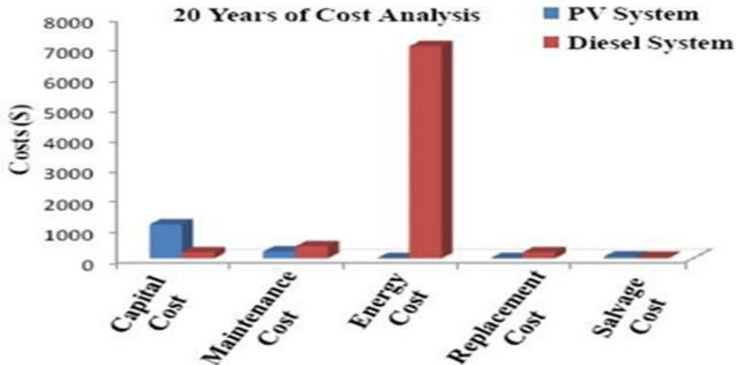
Figure 4. Cost Comparison PV and Diesel Systems [11]
