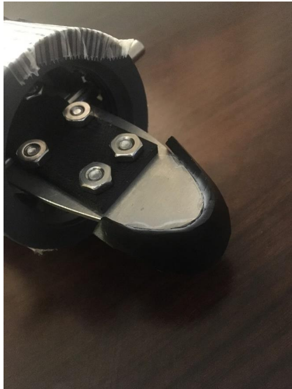
Figure 4: Rubber Shoe attached to the Valve
