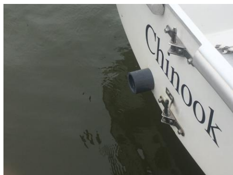
Figure 5: Stern level during unweighted stationary test
