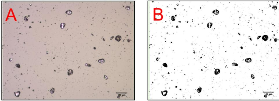
**FIGURE 8.** *A. bismuth telluride at 10x magnification. B. the powder post-process, as a black and white mask*
