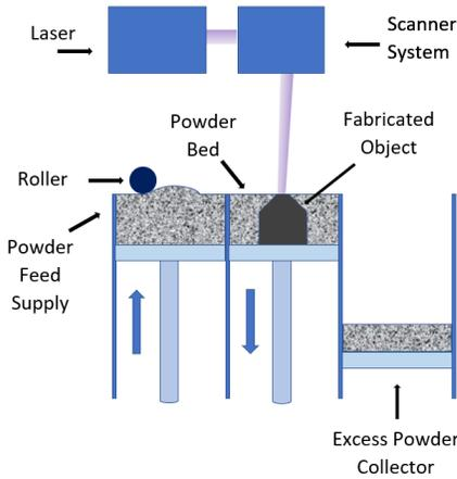
**FIGURE 3.** Schematic of Selective Laser Melting approach, eliminating dicing and assembly steps, and allowing desired geometries (Leinenbach, n.d.)
