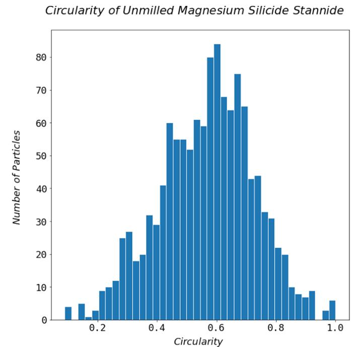
**FIGURE 9.** *A graph of the overall circularity values, the average being around 0.6*
