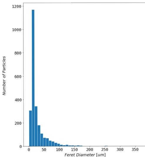
**FIGURE 10.** A graph of overall particle size distribution. Particles ranged from 5 $\mu$ m to 375  $\mu$ m, with the average being around 25 $\mu$ m.
