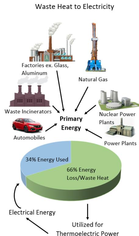
**FIGURE 1.** | Examples of heat and combustion systems which on average lose 66% of their energy to waste heat (Joly et al., n.d.)
