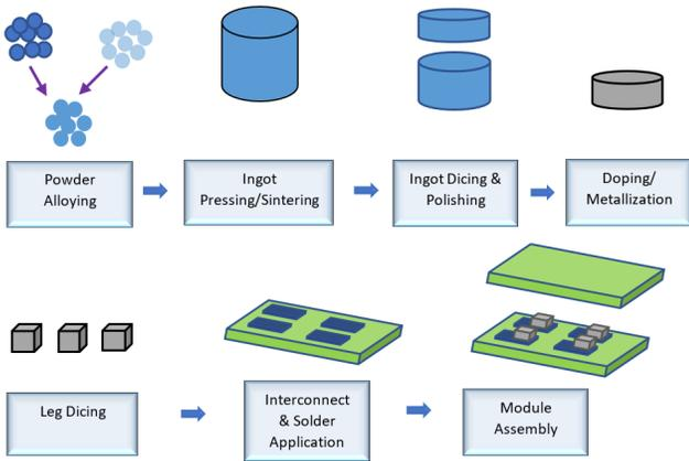
**FIGURE 2.** Typical steps for traditional manufacturing of thermoelectric devices (LeBlanc, 2014)
