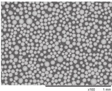
**FIGURE 4.** Image of optimal powder profile: high values of circularity, convexity, and desired powder distribution (Triantaphyllou, Giusca, Macaulay, Roerig, Hoebel, Leach, Tomita, and Milne, 2015)
