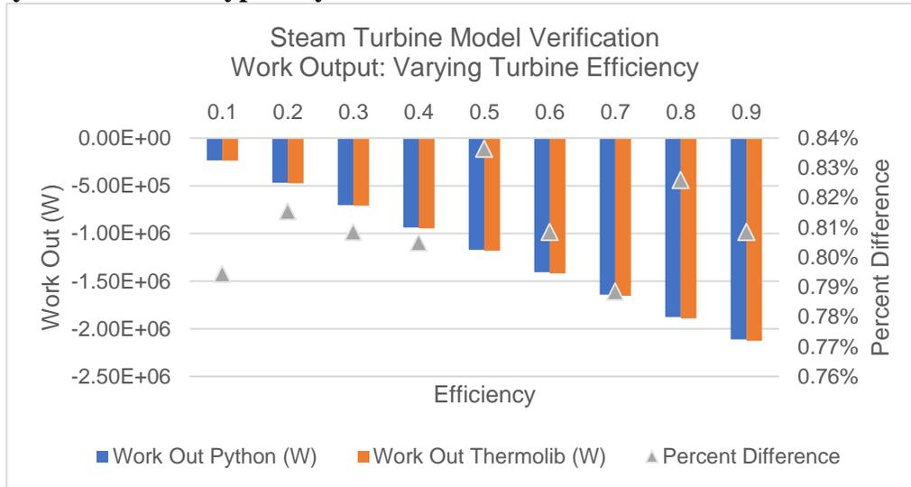
Figure 6: Steam Turbine Model Verification - Work Output Varying Turbine
