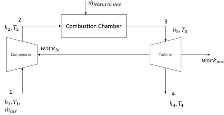
Figure 4: Brayton Cycle diagram of the CGT
