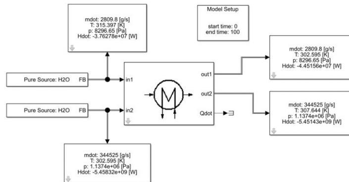
Figure 7: Condenser Simulink Simulation Results
