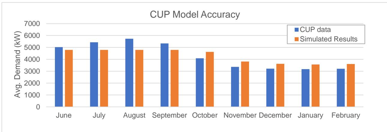
Figure 9: CUP Model output compared to actual CUP output. The maximum output of the model is limited to 4.7 MW.
