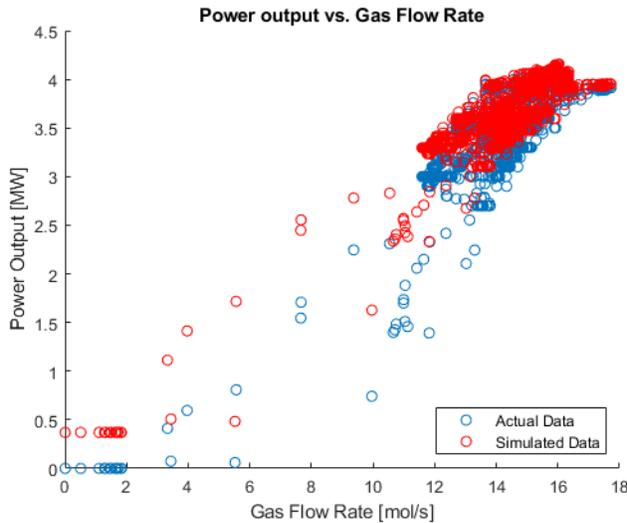
Figure 8: Simulated power output plotted against gas flow rate and compared to the actual demand and flow rate for the CUP gas turbine.
