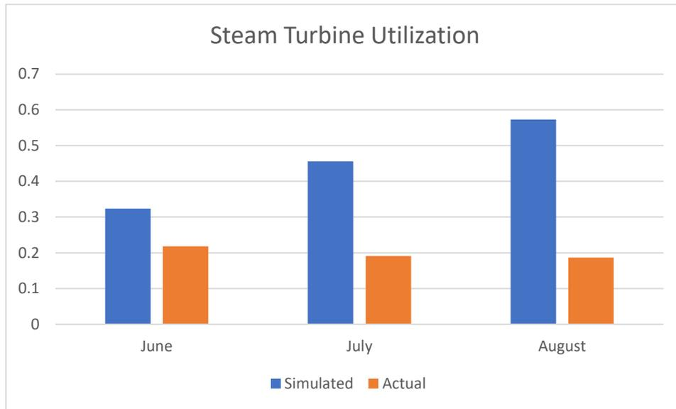
*Figure 11: Utilization change of the steam turbine with a steam bypass system for the summer of 2018.*
