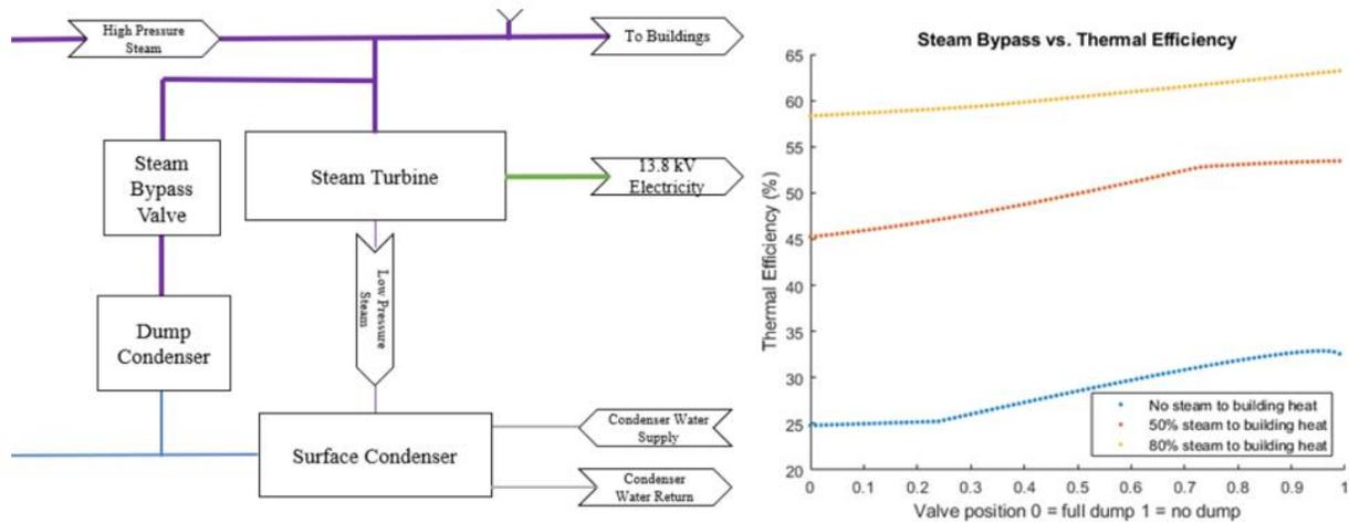
Figure 10: Steam Bypass system and dump condenser (left) and thermal efficiency change with bypass system valve position (right).
