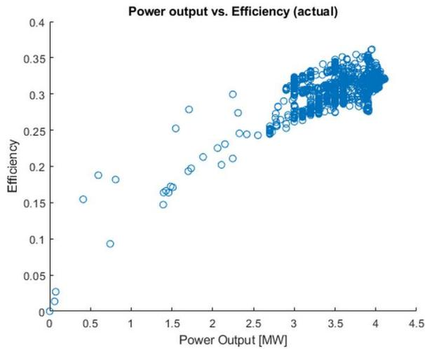
Figure 2: CGT Power vs. Overall Efficiency
