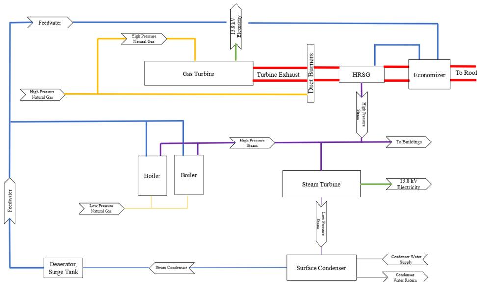
Figure 1: CUP simplified schematic.
