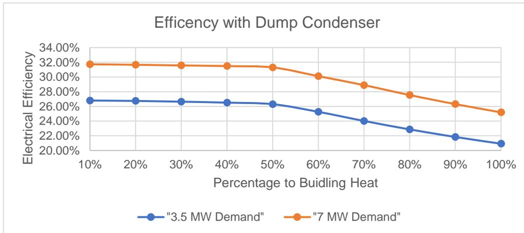
Figure 12: Model change in electrical efficiency with dump condenser with varying power
